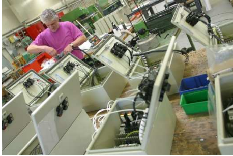
Batch production of valve control systems for the shipbuilding industry
